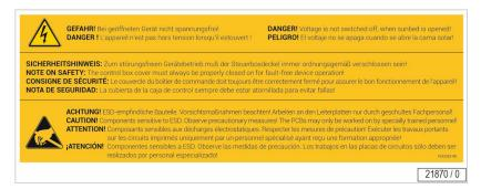
The sticker is mounted on the controller support.
