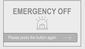
When the EMERGENCY OFF button is pressed, the entire unit apart from the INTERIOR DISPLAY switches off. In this state, a display appears to show that the EMERGENCY OFF button has been operated.
