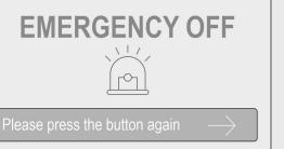
When the EMERGENCY OFF button is pressed, the entire unit apart from the INTERIOR DISPLAY switches off. In this state, a display appears to show that the EMERGENCY OFF button has been operated.
