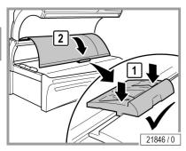
Carefully lay the panel aside on the scratch protection (service kit).
