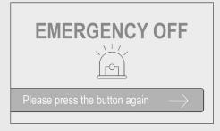
When the EMERGENCY OFF button is pressed, the entire unit apart from the INTERIOR DISPLAY switches off. In this state, a display appears to show that the EMERGENCY OFF button has been operated.
