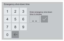
Enter the emergency shut-down time via the keypad; the time
