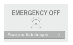
When the EMERGENCY OFF button is pressed, the entire unit apart from the INTERIOR DISPLAY switches off. In this status, the display shows that the EMERGENCY OFF button has been operated.
