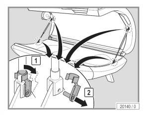
Remove the gas pressure absorber
