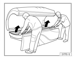
Remove the acrylic panel and carefully lay it aside.
