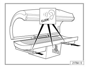
Re-insert the cleaned and dried filter. The two outer filter must audibly click into place.
