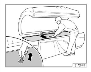
Push the bed to the rear with one hand and pull it out of the front guide with the suction cup.
