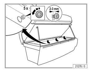
Loosen 5 screws (do not remove):
