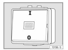
The electrical installation must have a freely accessible, all-pole disconnecting device (Master switch with clearly labelled On/Off settings, e.g. '0' and 'l' or additional indicator light) fitted externally on the site.
