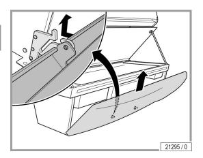
Remove the front panel from the guide.
