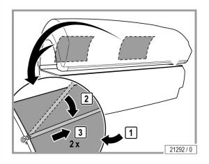
Reinstall the cleaned and dried filter mat.
