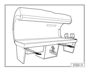
Pull out the two outside filters to the front. Remove the middle filter via the top.
