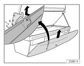
Remove the front panel from the guide.
