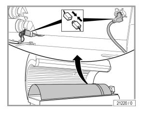
The canopy panel must be completely removed from the device in order to replace the low pressure lamps.
