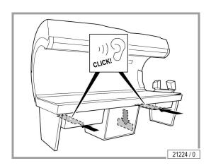
Replace the cleaned and dried filters. The two outer filters clip into place with an audible click.
