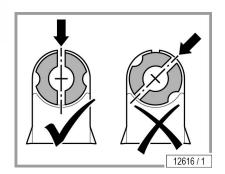
Before inserting the new lamp, the alignment of the inner part of the socket must be checked.
