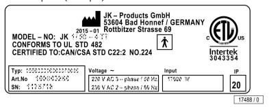
The name plate is attached to the interior side of the canopy. It contains important information for identifying the device (e. g. the serial number = Serial-No.) and the conformity mark.
