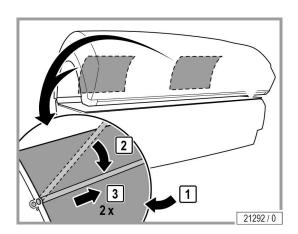
Reinstall the cleaned and dried filter mat.
