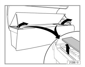
Remove the lamp covers at the head and foot ends.
