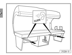
Re-insert the cleaned and dried filter mats. The two outer filter mats must audibly click into place.
