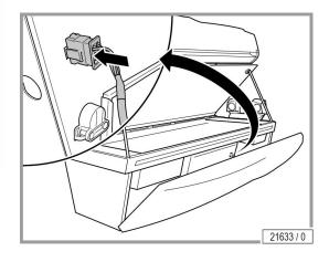
– Plug connector ST 54 into the part carrier.
