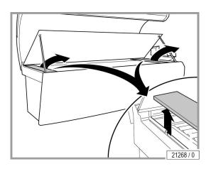
Remove the lamp covers at the head and foot ends.
