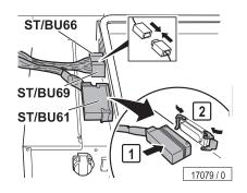
– Plug in connectors on the left side of the component rack.
