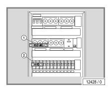
In case of circuit breakers which cannot be unscrewed, a strip of adhesive tape may be applied over the actuation lever with the wording 'Do not switch, danger!' (1 + 2).
