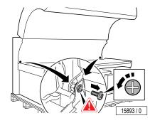
Remove the left and right side screws.
