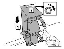
Suspend AQUA / AROMA SYSTEM into recess and tighten screw.
