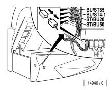
Plug in connectors at the base end (control unit).
