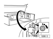
Re-fasten the side panel safety switch holding bracket.
