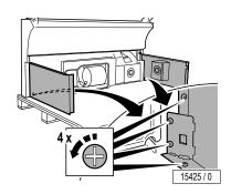
Tool: No. 2 Philips screwdriver or battery-powered screwdriver with PHZ-bit 2
