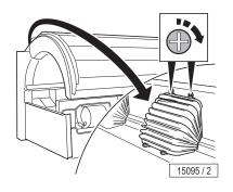
Hook in bellows and tighten screws.
