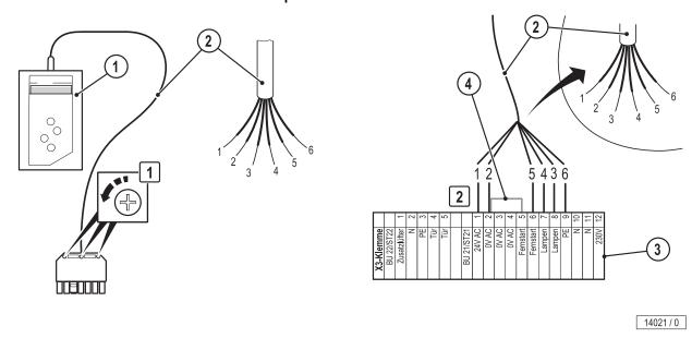
The plug on the manual control unit (1) must be dismantled. The control line (2) is directly connected to the connector strip (3) of the device.
