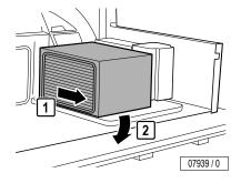
Slightly lift air conditioning unit and and put on front left border edge.
