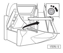
Fasten the metal sheet for electrical grounding to the front panel.
