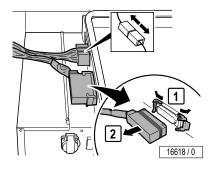
Unplug remaining connectors on the left side of the component rack.
