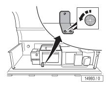
Unscrew the screws of the component rack transport lock.
