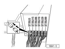
Plug in connectors at component rack.
