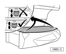
The magnets must be in contact.
