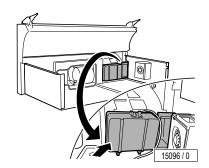
Carefully insert ventilation duct diagonally to the back and press in front.
