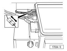
Unplug the rear two connectors on the left side of the component rack.
