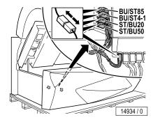
Unplug plug connections at the foot of the device (control unit).
