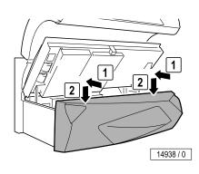
Refit the front panel and then press it downwards until it latches into place.
