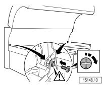
Fasten left and right screws through the support with bushings.
