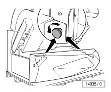
Unscrew and remove both knurled thumb-screws that hold the front panel in place.
