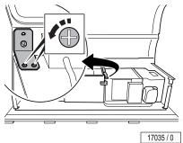
Unscrew the holder between air conditioning unit and component rack.
