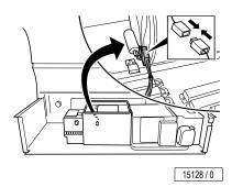
Plug the connector into the device fan.
