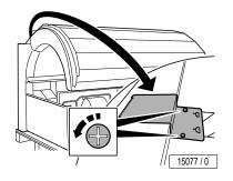
Unscrew the cable duct covering and remove it.
