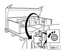
Unscrew side panel safety switches' holding bracket.
