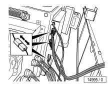
Unplug all plug connections from the box at the front of the component rack.
