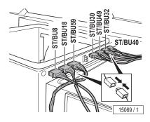
Plug in all connectors on the right side of the component rack.
