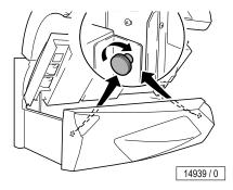
Retighten the knurled thumb-screws that hold the front panel in place.
